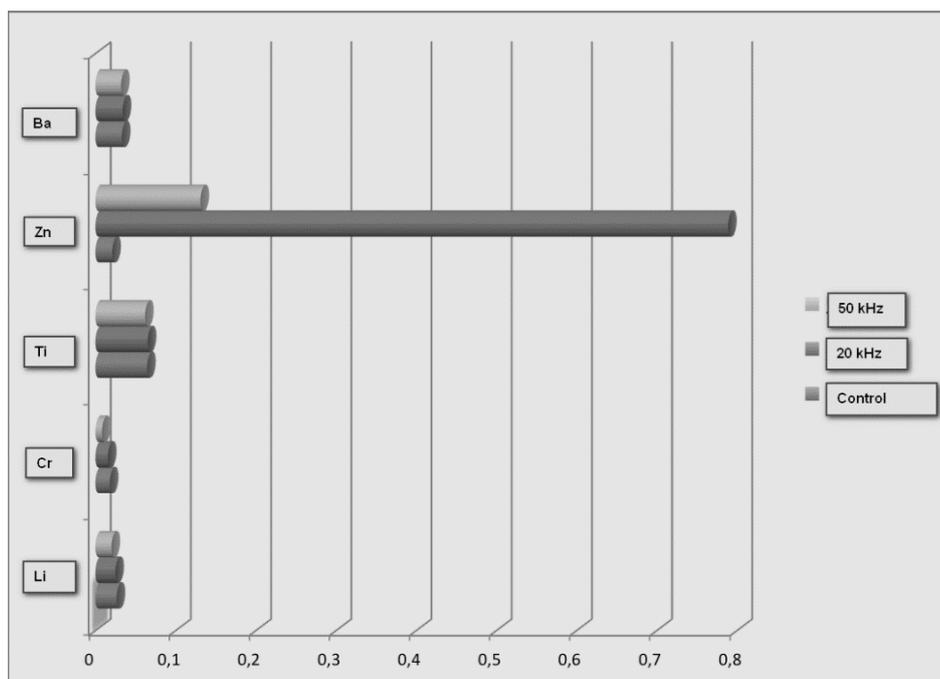
**Fig.4.** The increasing of Zn concentration in water after ultrasound influence.
