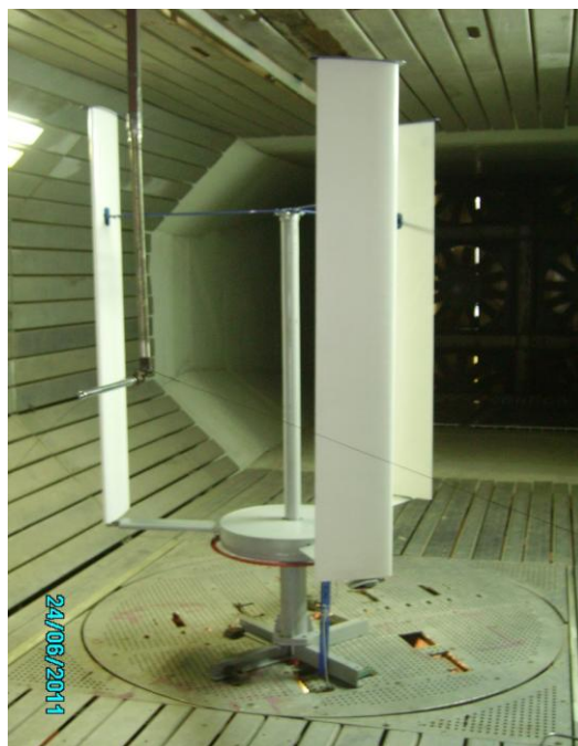
Fig.1. The wind turbine with controlled blades in the wind tunnel
