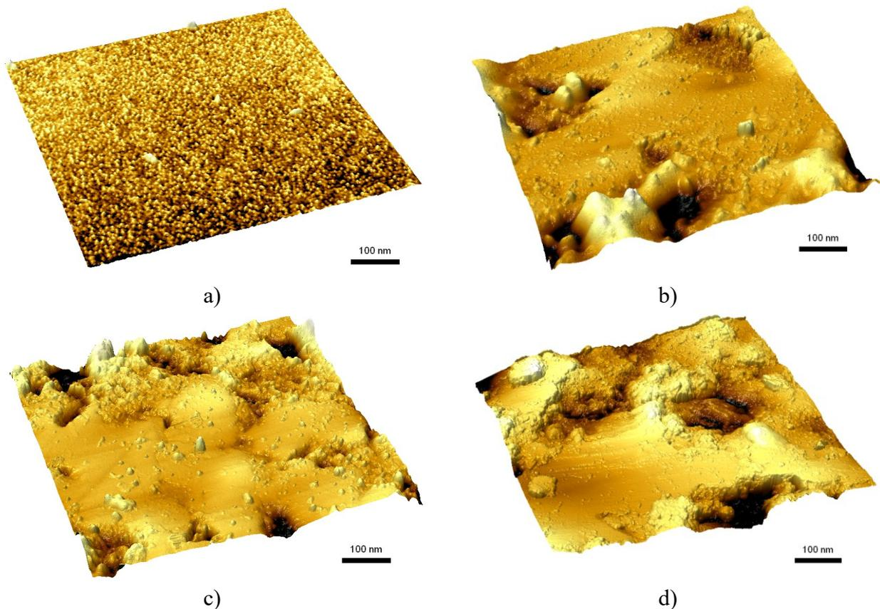
**Fig.2.** 3D atomic force microscopy (AFM) images of ceramics before and after irradiation:
